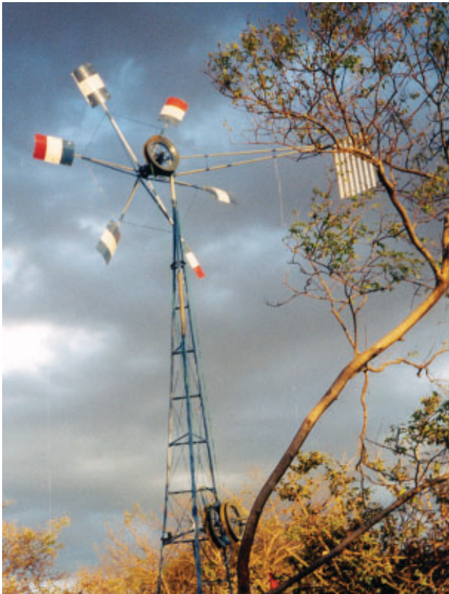
Windmill in Nicaragua. Wind energy does not have to be high-tech: in many developing countries simple windmills are used for pumping water.
