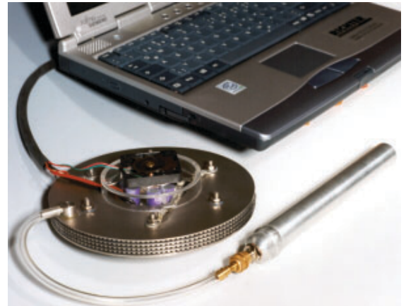
A small fuel cell powering a laptop. The thin cylinder holds the hydrogen.
